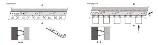
• Panels are removed by peeling the panel edges from the prongs of the carrier and sliding the panel out of the slot.
