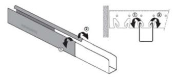
• Carrier splices are removed by squeezing the vertical flanges of the carrier just below the carrier splice until the lips in the splice disengage from the holes in the carrier side. The splice can then be easily lifted off.
