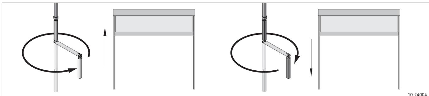
**⚠** Do not try to further continue operating the external roller blind when there is more than normal resistance, through the mechanical limitation. The resistance to be met is subjective, however the force required is a maximum of 40N (approx. 4kg).
