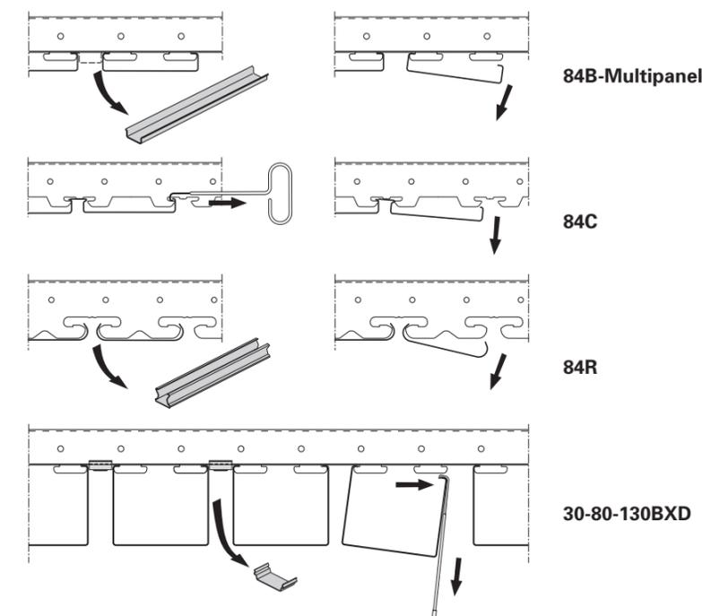
**GB** While demounting the panel make sure to support the part of the panel that has already been removed from the carriers.
