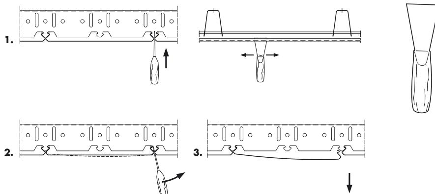
**GB** Demounting the panels shall only be done utilising a putty knife. Any other tool may damage the panels. While demounting the panel make sure to support the part of the panel that has already been removed from the carriers.
