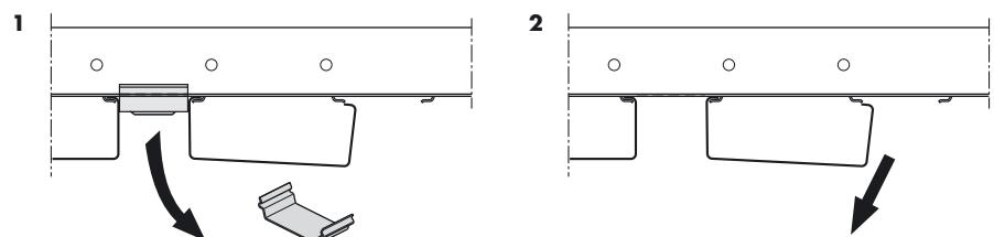
**GB** While demounting the panel make sure to support the part of the panel that has already been removed from the carriers.
