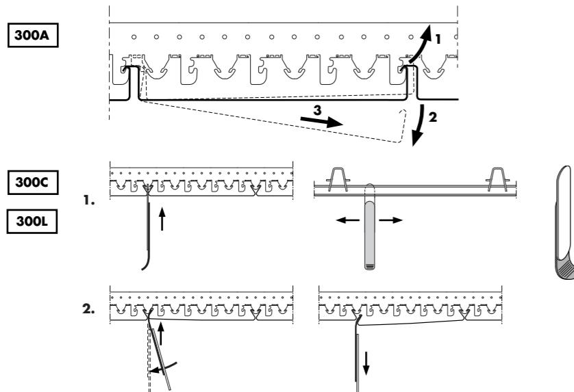
**GB** Demounting the panels shall only be done utilising the special demounting tool. Any other tool may damage the panels. While demounting the panel make sure to support the part of the panel that has already been removed from the carriers.
