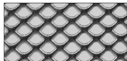
LS10 Fe open area 68%, thickness 2.0 mm
